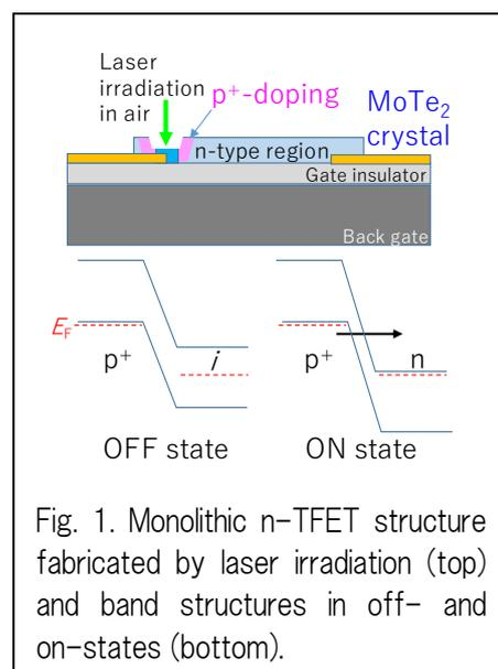
Fig. 1. Monolithic n-TFET structure fabricated by laser irradiation (top) and band structures in off- and on-states (bottom).
